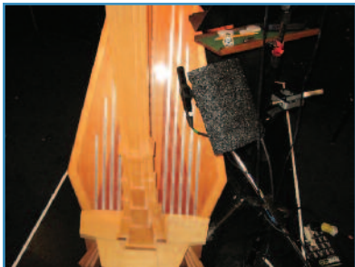
The screen is fixed to a slim 12" gooseneck with three small fasteners.
